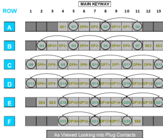
Figure 13.5.2.8-1: J7-High Speed Electrical Connector Pin Arrangement
