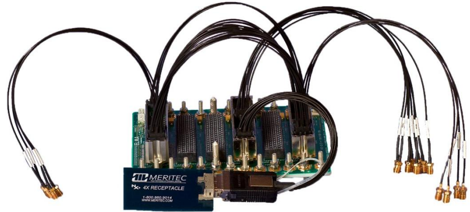
Fat Pipe – CX4 Ultra Thin Pipe – SMAs Fat Pipe from RJ1 to RJ6
